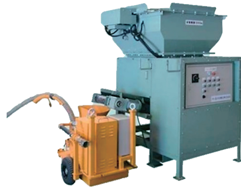
Fig. 5 Exterior view of gunning machine of gunning plastic refractory.
